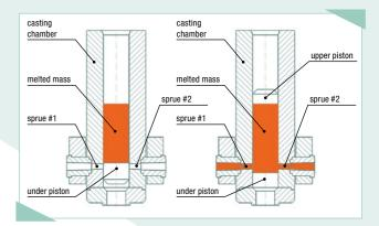
The vertical arrangement provides a 100% filling rate of the casting chamber and eliminates the known problems of air pockets during the 1st phase of the mould filling process. Next to this, the closing of the gates during the dosing process provides an optimal chance to evacuate the two moulds.
